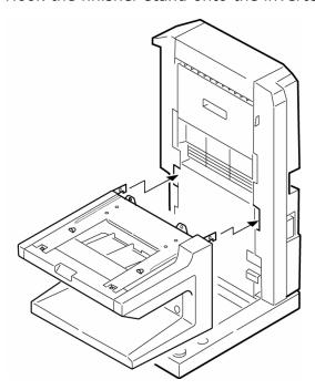
2. Attach the finisher stand to the inverter with 2 screws.
